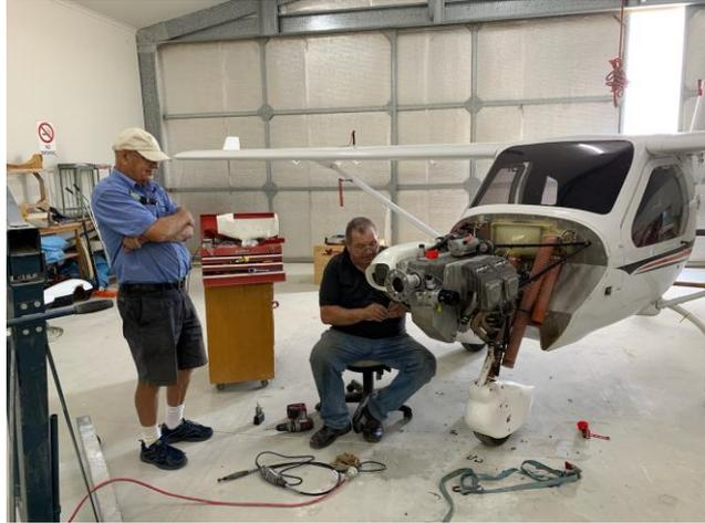
The newest Jabiru in our fleet, 8538, has proven to be so popular that its engine has reached its TBO hours in just over 2 years. A new Generation 4 Jabiru engine has been installed into 8538. Thanks for your hard work here Mick! (With Karl keeping a close eye on things of course!!)
