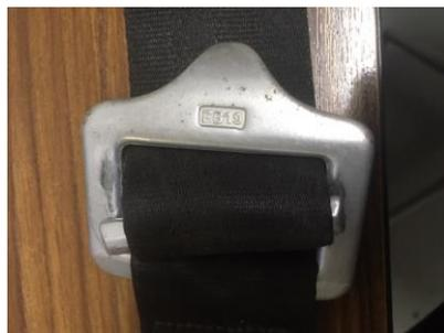
The buckle end strap was removed from the adjuster, and the spring was removed and inspected for damage. No damage was found and the spring was securely refitted. Paul reported that the spring is a firm fit and is working as intended. The reason why the spring came loose was not identified.
