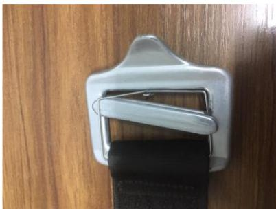
While on a high-speed final glide to Gawler, a Discus flew through some rough turbulence. The left-hand hip strap of the harness came loose and the pilot struck their head on the canopy. Attempts by the pilot to tighten the strap proved fruitless, and it kept coming loose. The pilot reduced speed to minimise the effect of the turbulence and landed safely.
