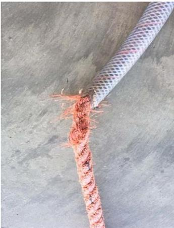
Clearly this rope is unserviceable and should have been condemned.
