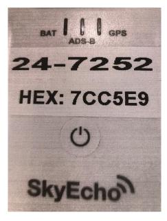
When the unit is working correctly – the GPS and ADS-B lights will blink green.
