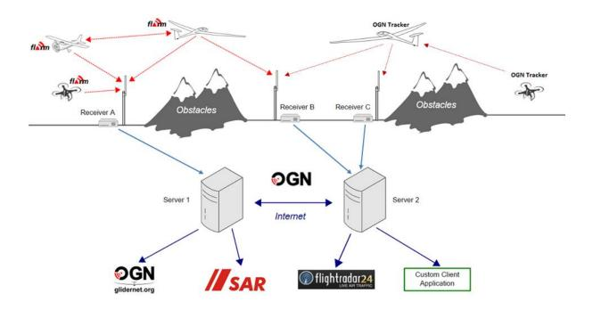
This system for displaying glider traffic on OzRunways will only display glider that are in the coverage area of the OGN receivers. There are currently OGN receivers at YBVA (Balaklava), YGAW (Gawler), YSFG (Stonefield), and YWKI (Waikerie).
