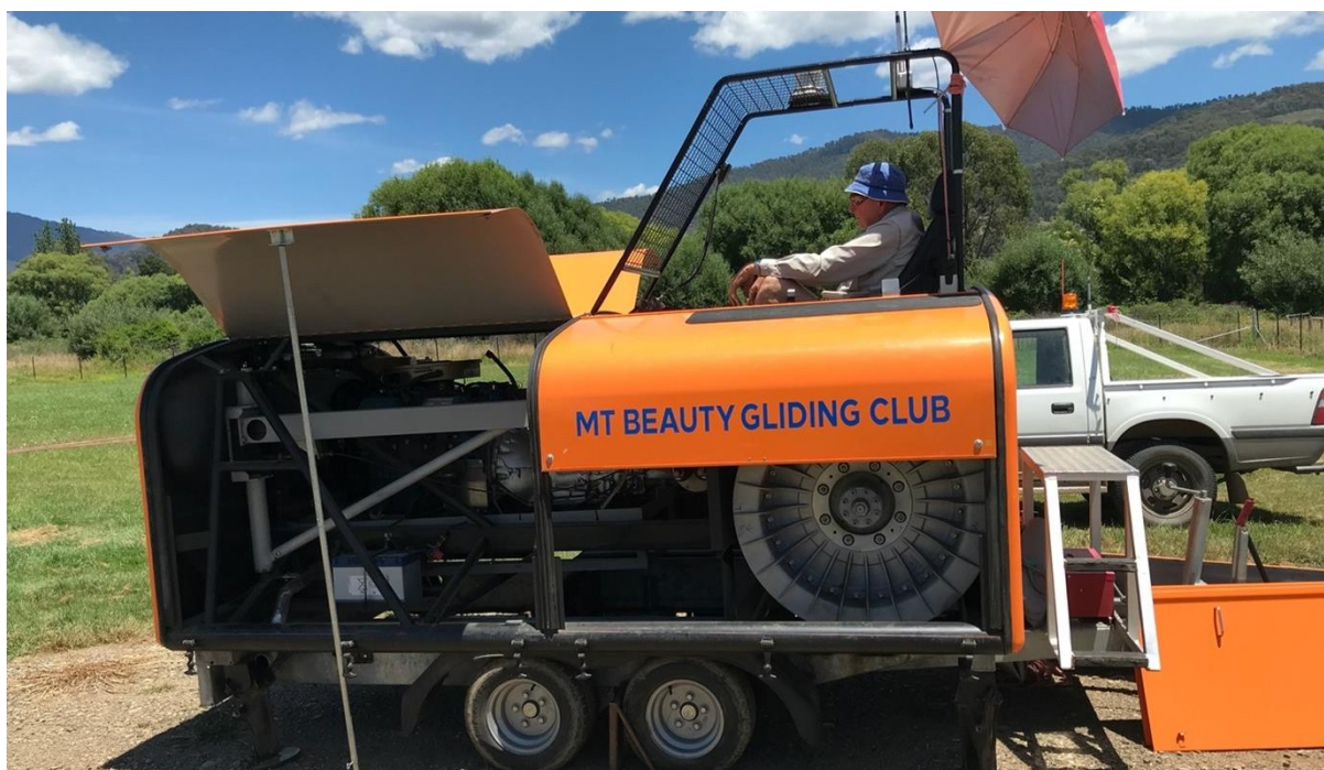
Gliders are launched using this fixed site TOST winch.
